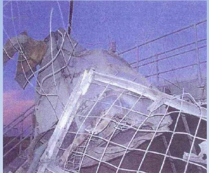
Photo 1.6 Fan Cowl Lodged in the Explosion Door Opening
